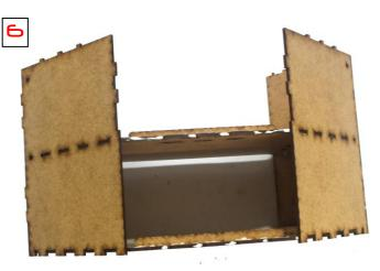
6 Glue on the 2 back / side walls, and ensure that the whole module is straight. Tabs sticking out the bottom is correct.
