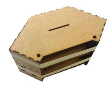
8 Glue on the top plate. Best to hold together with masking tape during glue drying time, so that the center back plate sits properly. Ensure proper angles.
