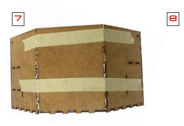
7 Glue on the large center back wall with plenty of glue between the angled pieces to ensure they hold properly and the gaps are closed.
