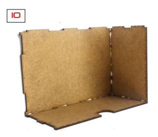
**10 Drawers:** glue a sidewall and front wall to the base plate.
