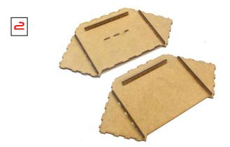
2 first glue in 3 of the drawer limiters into the bottom and middle large plates.
