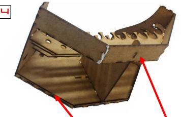
4 then glue in the 3 slim strips at the bottom and the 3 larger ones at the top. Make sure to put plenty of glue between the large ones to close the gap of the angles.
