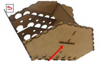
5 Glue in the slim strip with 3 tabs into the slots from the bottom. Careful not to break it. The strips from 4 stick out at the bottom. This is correct.
