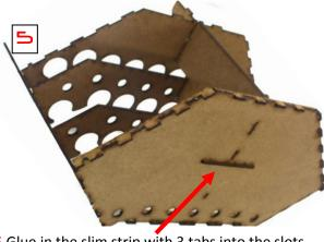
5 Glue in the slim strip with 3 tabs into the slots from the bottom. Careful not to break it. The strips from 4 stick out at the bottom. This is correct.
