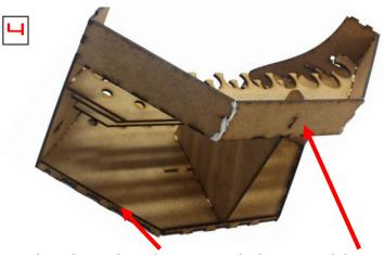
4 then glue in the 3 slim strips at the bottom and the 3 larger ones at the top. Make sure to put plenty of glue between the large ones to close the gap of the angles.
