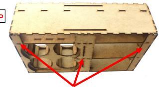
6 glue on the upper plate, then the 3 support strips at the back, round cutouts where the spray cans are. Ensure right angles.
