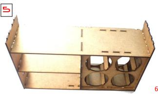
5 glue on the 2 sidewalls, tabs to the back.
