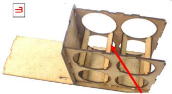
**3** Glue this into the bottom plate. Glue in all the support strips into the cutouts of the spay can holders.
