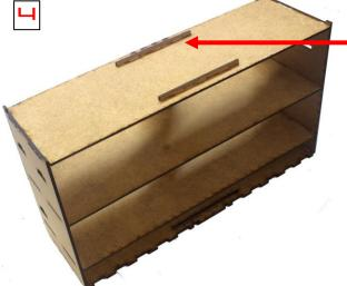
4 Glue in the 2 small strips with the 3 tabs into the slits of the bottom from below
