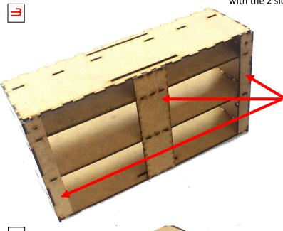
3 glue on the top plate. Then glue on the 3 support strips at the back. Ensure right angles.
