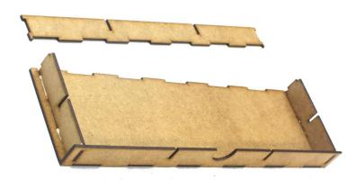
2 first glue in the 2 sidewalls into the slits of the bottom. Then glue in the front wall.
