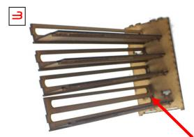
3 glue the paint holders into one sidewall. The one with 2 slits at the bottom. Ensure right angles.
