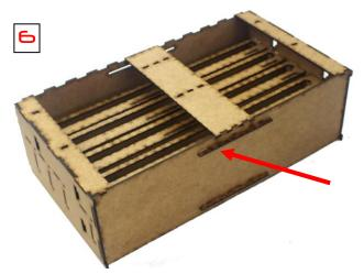
6 glue on the upper plate, then the 3 support strips at the back. Ensure right angles. Also glue in the 2 small strips with the 3 tabs into the slits of the bottom from below.
