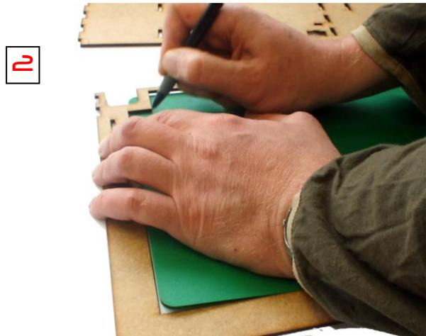
**2** first place the cutting mat fitting into a frame and mark the corners. Cut these corners out of the cutting mat with strong scissors or a sharp blade.
