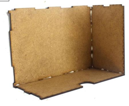
**Drawers:** glue a sidewall and front wall to the base plate.
