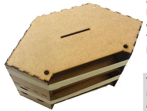
8 Glue on the top plate. Best to hold together with masking tape during glue drying time, so that the center back plate sits properly. Ensure proper angles.
