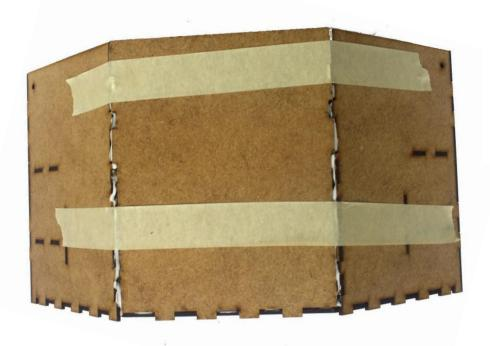
7 Glue on the large center back wall with plenty of glue between the angled pieces to ensure they hold properly and the gaps are closed.
