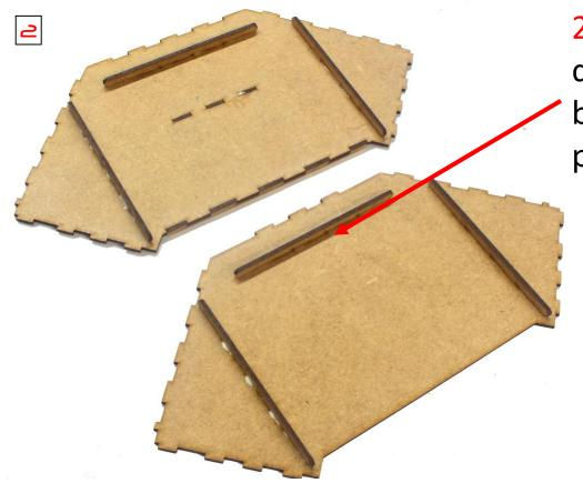
2 first glue in 3 of the drawer limiters into the bottom and middle large plates.
