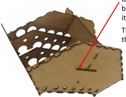
5 Glue in the slim strip with 3 tabs into the slots from the bottom. Careful not to break it.
