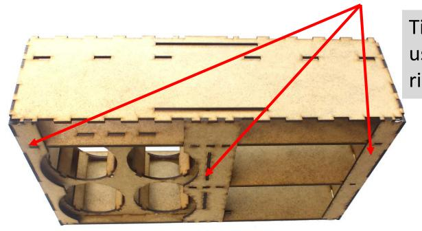
Tip: During glue drying use vice grips to ensure right angles / fit.
