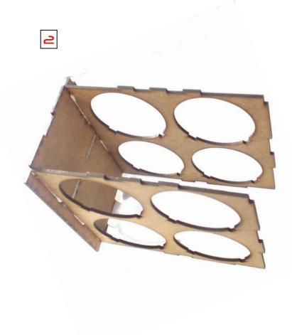
2 first glue in the 2 spray can holders into the slits of the middle wall.
