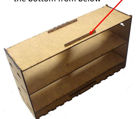
Tip: During glue drying use vice grips to ensure right angles / fit.
