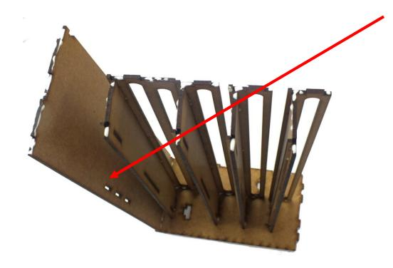
4 Glue in the bottom plate, tabs facing the back.
