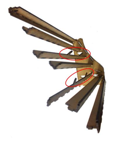
4 glue the pieces of group 1 and 2 into the slots of a sidewall as shown.
