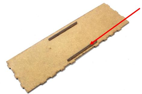
2 first glue in the 2 small strips with the 3 tabs into the slits of the bottom from below.
