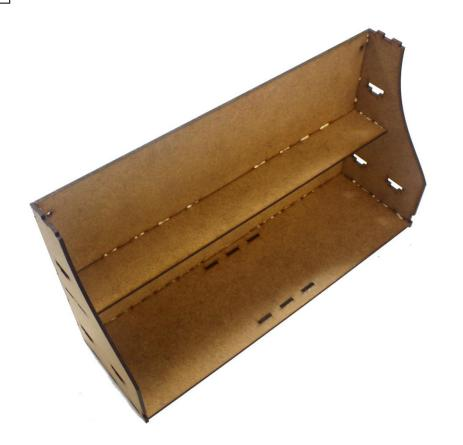
Tip: During glue drying use vice grips to ensure right angles / fit.
