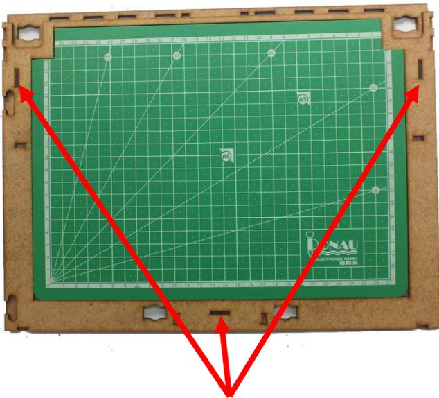
Tip: weigh down with around 20 KG of weights during glue drying time, so that there are no gaps between the layers!
