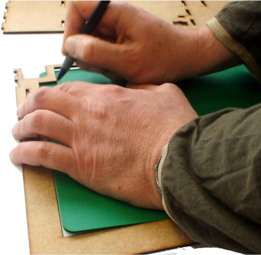
2 first place the cutting mat fitting into a frame and mark the corners.
