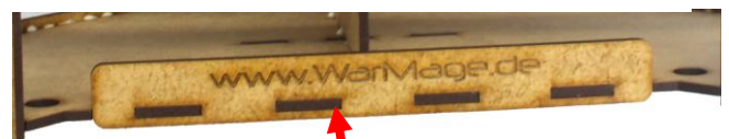
6 Glue the front support strip (4 slits) onto the front of the base plate, and ensure that the whole module is straight. Also glue the little piece with 3 tabs into the slits of the bottom plate from below.
