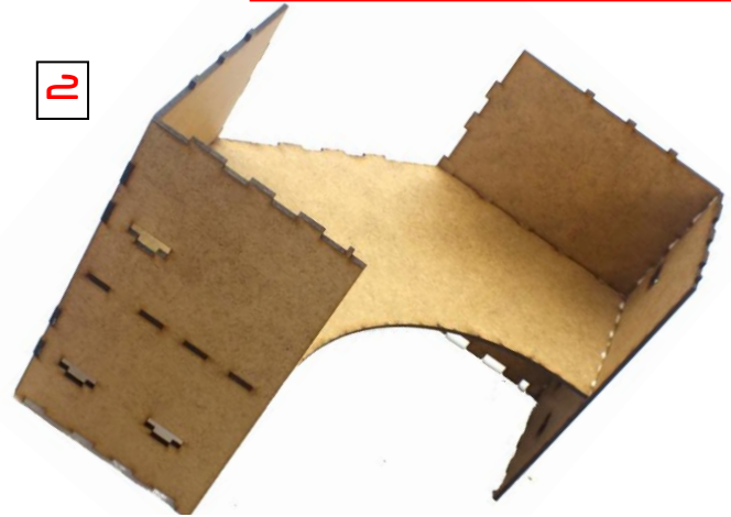
2 first glue in the middle shelf into the 2 sidewalls and 2 back walls.
