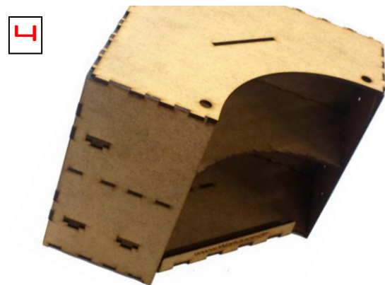
4 then glue in top plate (with 2 round holes in it)
