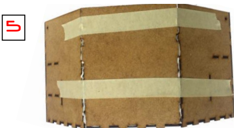
5 Glue on the large back wall with plenty of glue between the angled pieces to ensure they hold properly and the gaps are closed.
