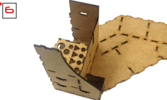
6 Glue on the side wall, tabs all fully inserted.
