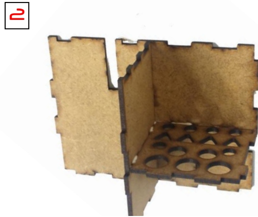
2 first glue in one brush holder into the middle wall and glue these 2 into the front wall, as in the picture.
