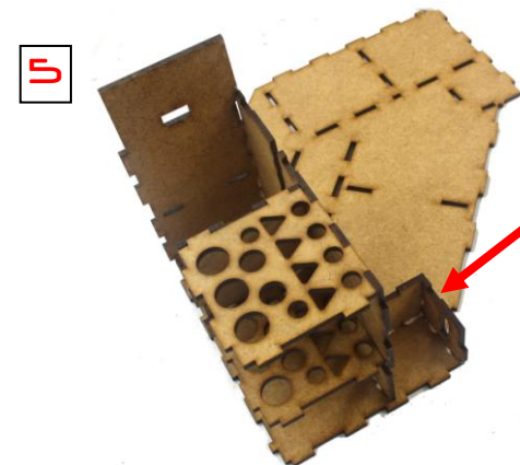
5 little pieces: the one WITH hole towards the front! These are a little tricky to glue in the slits.
