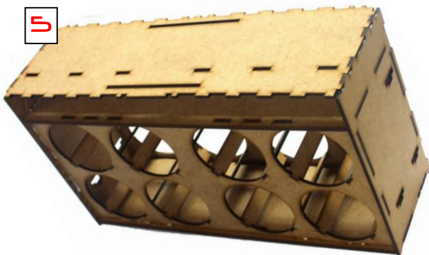
5 glue on the other sidewall and the top plate.
